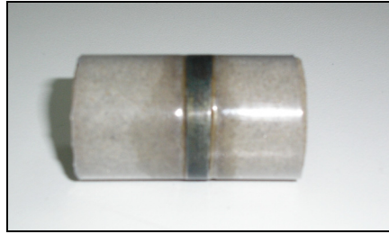
Figure 1: In-house developed specimen used for permeability experiments.
